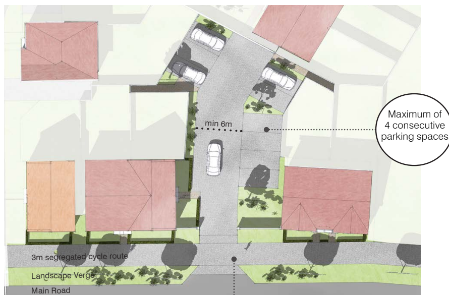
Figure 6.39: Proposed rear courtyard parking arrangement
