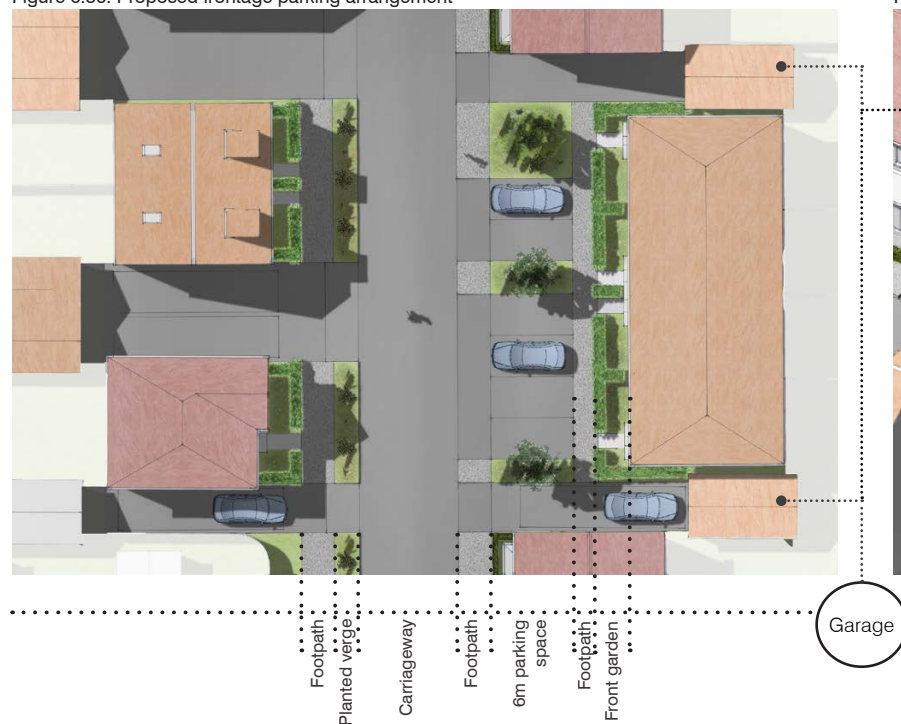
Figure 6.36: Proposed frontage parking arrangement
