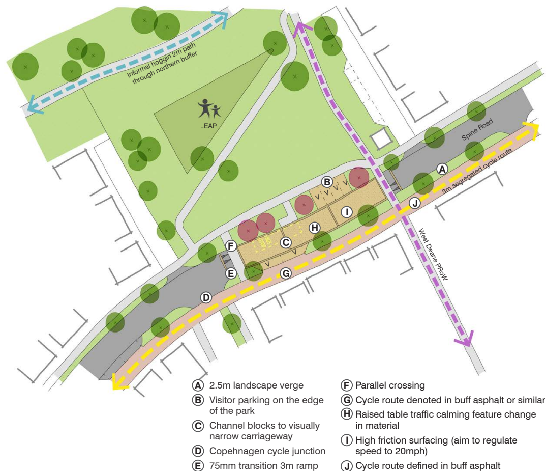
Figure 6.32: Illustrative layout highlighting highway design components to achieve traffic calmed nodal areas
