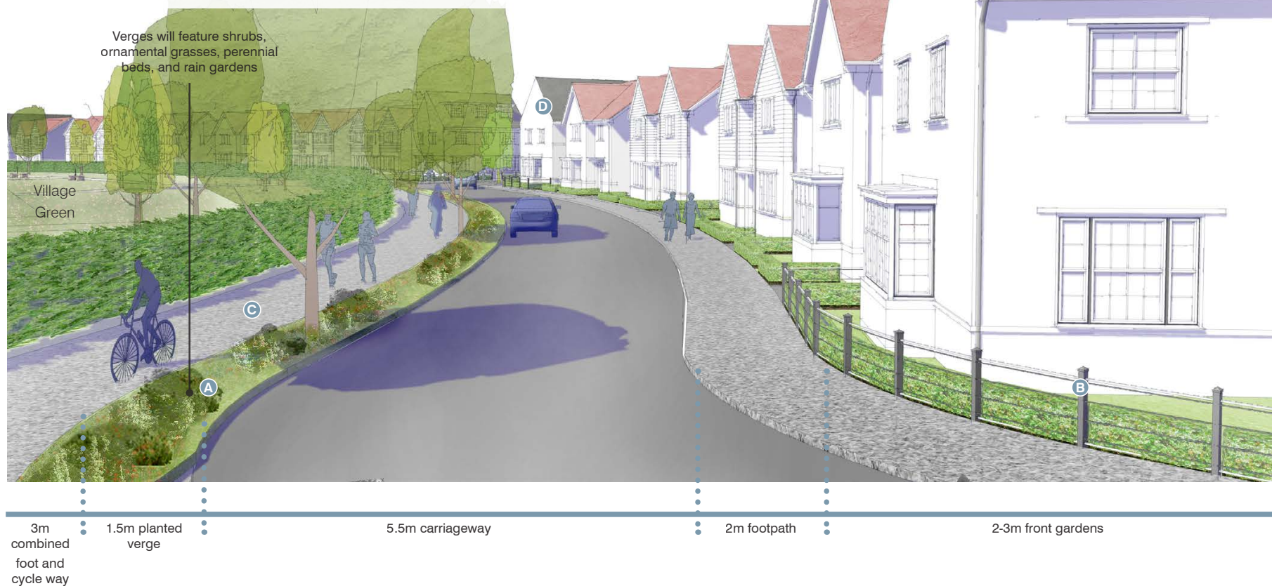
Figure 6.07: Green Street Section
