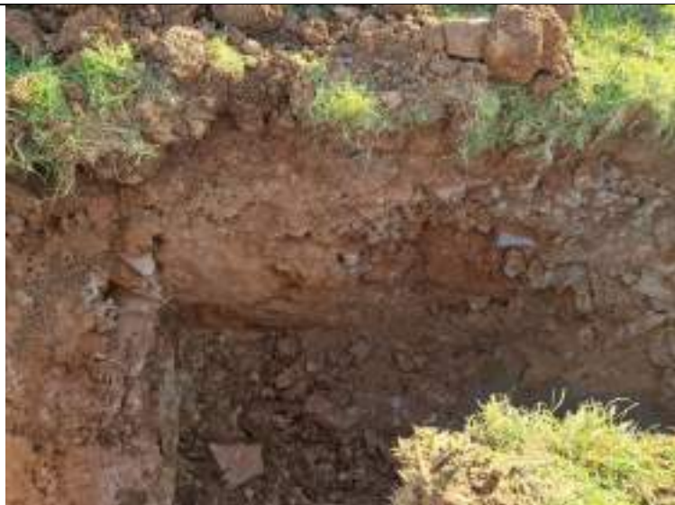
PLATE 01 – Trial Pit Excavation – TP01.
