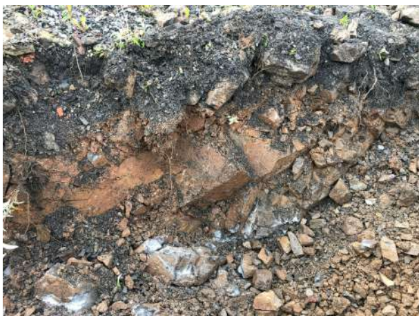
Photo 3: A view of the sidewall from SA02 showing minimal Made Ground overlying very shallow limestone bedrock fractured and locally oxidised.
